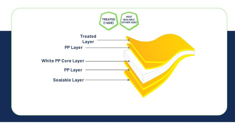
Application: White CPP film, which is used as a single ply or lamination layer wherever white color of film is an advantage for final applications, e.g. confectioneries, condiments, etc.
