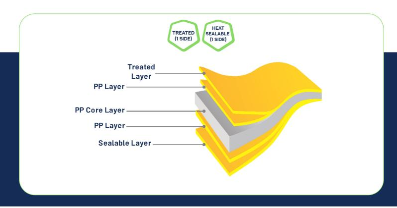
Application : General-purpose lamination CPP film with tight and strong sealing property for packaging applications, e.g. bread, pasta, etc.
