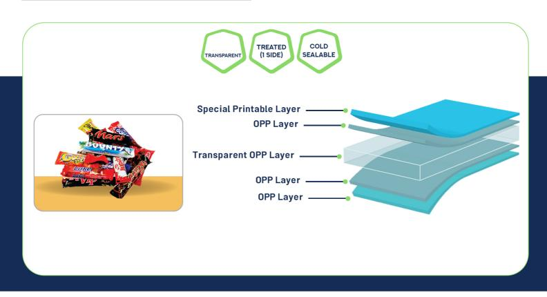
Application: Cold seal packaging applications. It can be used as printing substrate & lamination substrate to itself and to other films. PF-Polin 121 CP can be used as printing substrate for missing-dot-free printing.
