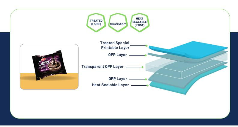
Application: General purpose packaging film for using on HFFS and VFFS machines. It can be used as single ply or as lamination substrate to itself and to other films. PF-Polex 321S can be used as printing substrate (for missing-dot-free printing) & lamination substrate to itself and to other films.
