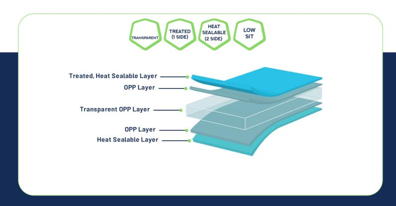
Application: General purpose packaging film for using on HFFS and VFFS machines. It can be used as single ply or as lamination substrate to itself and to other films. Heat sealing threshold of PF-Polex 221 D is lower than  $105\,^{\circ}$ C.
