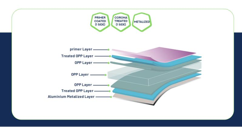
Application: Self-adhesive label (hot-melt or acrylic) production. This film can also be used for other kinds of applications such as cut & stack. Primer coated films are used for better printing.
