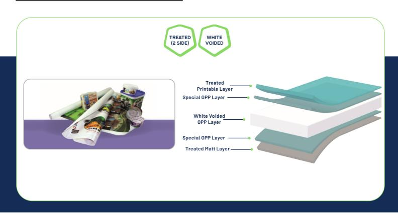
Application: In-mold labeling, suitable for sheet-fed and roll fed printing. This film can also be used for other kinds of applications such as cut & stack. It can be used instead of CPP IML films for rather big containers.
