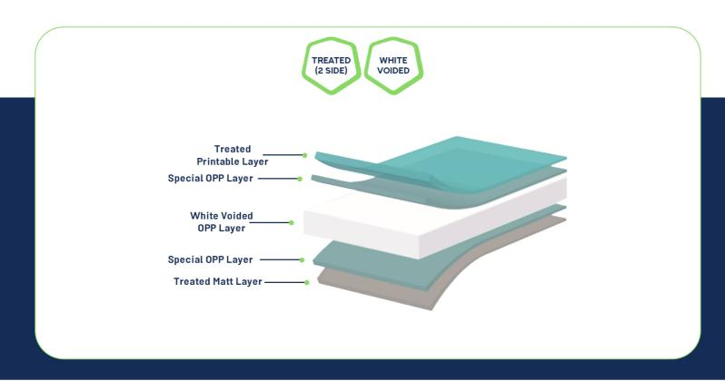
Application: High yield BOPP film for In-mold labeling, Specially designed for high speed sheet fed converting machine. This film can also be used for other kinds of applications such as cut & stack.
