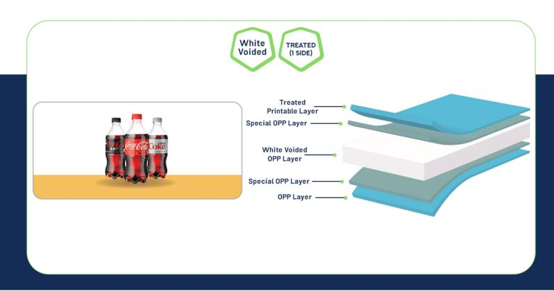
Application: White voided, opaque BOPP film, specifically developed for single ply roll-fed bottle labels. This film can also be used for other kinds of applications such as cut & stack.
