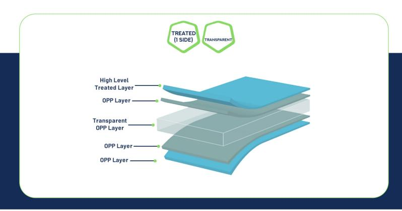
Application : For adhesive tapes. Treated side of this film is excellent for water based acrylic adhesive coating.
