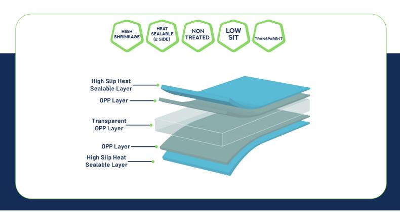
Application: Specially designed to be used on high speed over wrapping machines. This film has high shrink property to provide a tight wrap. Also It has a good antistatic property to prevent dust accumulation on film surface.
