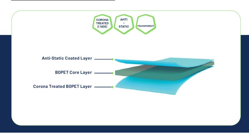
Application: Anti-static coated transparent Foldable film used for twist wrap packaging of confectionary products like candies, chocolates, etc. This film provides good anti-static properties for high speed packaging machines.
